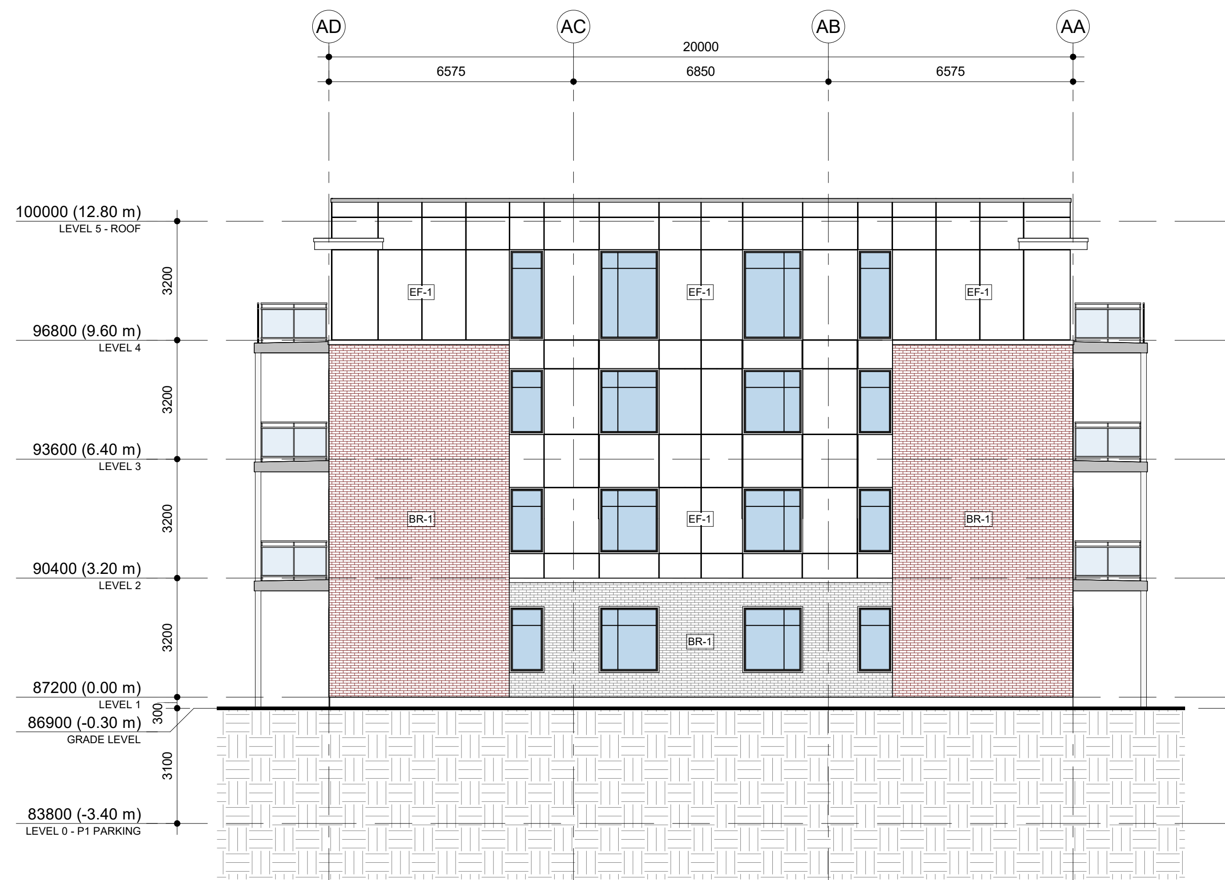
1 BUILDING A - NORTH ELEVATION A201 1 : 100
