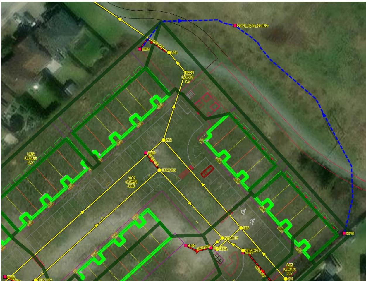
Figure 2 above presents a portion of the PCSWMM model which demonstrates the object connectivity. The subcatchment are illustrates as white polygons, with their area number, area in hectares and percent imperviousness labelled. The yellow lines and circles represent the storm sewer system and manholes, with red dashed lines representing the OUTLET links (or ICDs). The dashed blue lines represent the major
