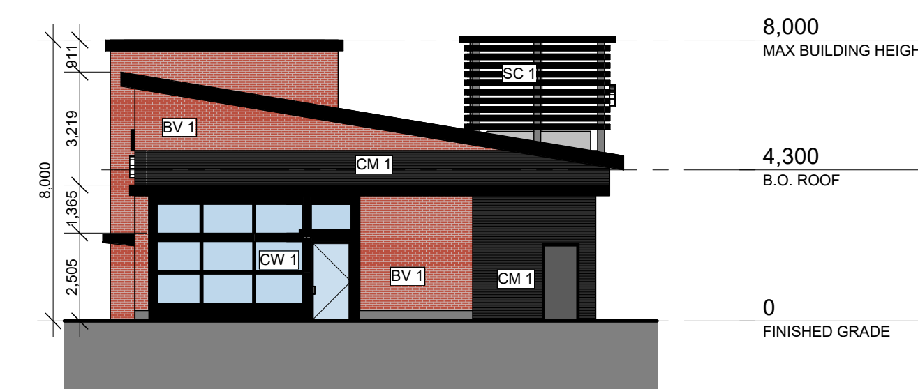
3 BUILDING F - WEST ELEVATION 1:150
