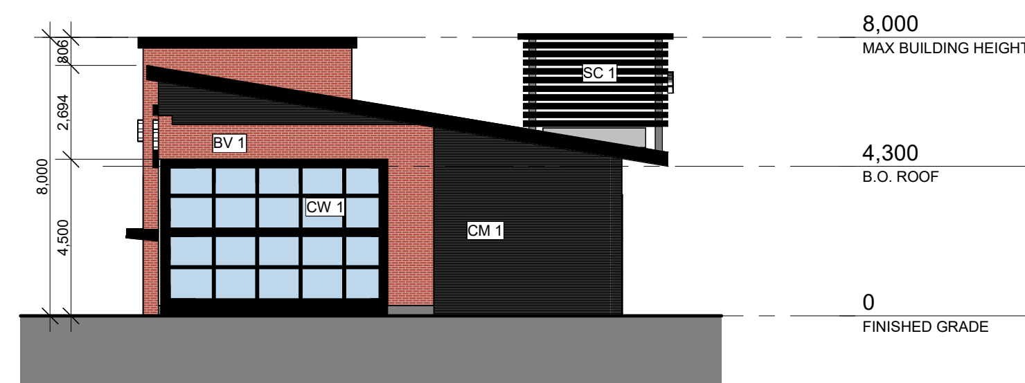
2 BUILDING B - EAST ELEVATION 1 : 150
