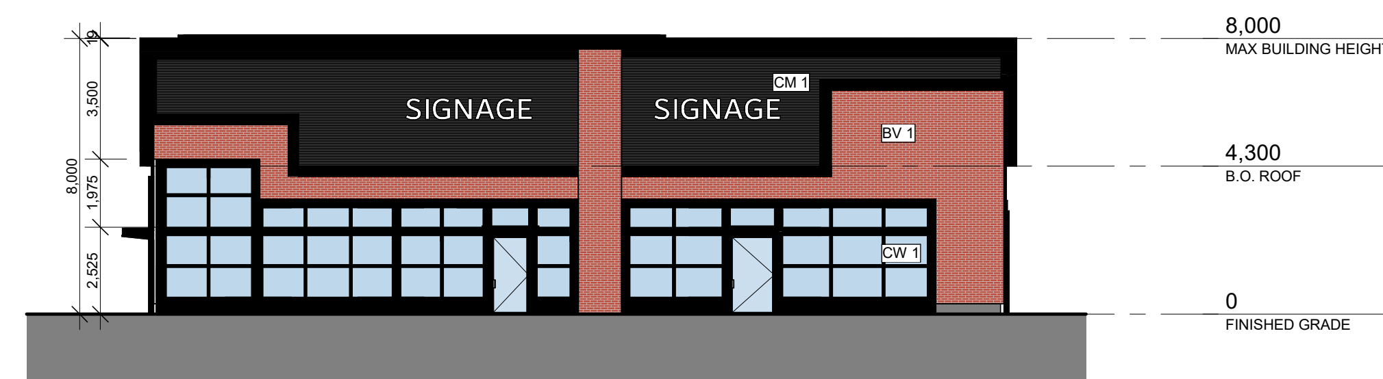
1 BUILDING C - SOUTH ELEVATION 1:150
