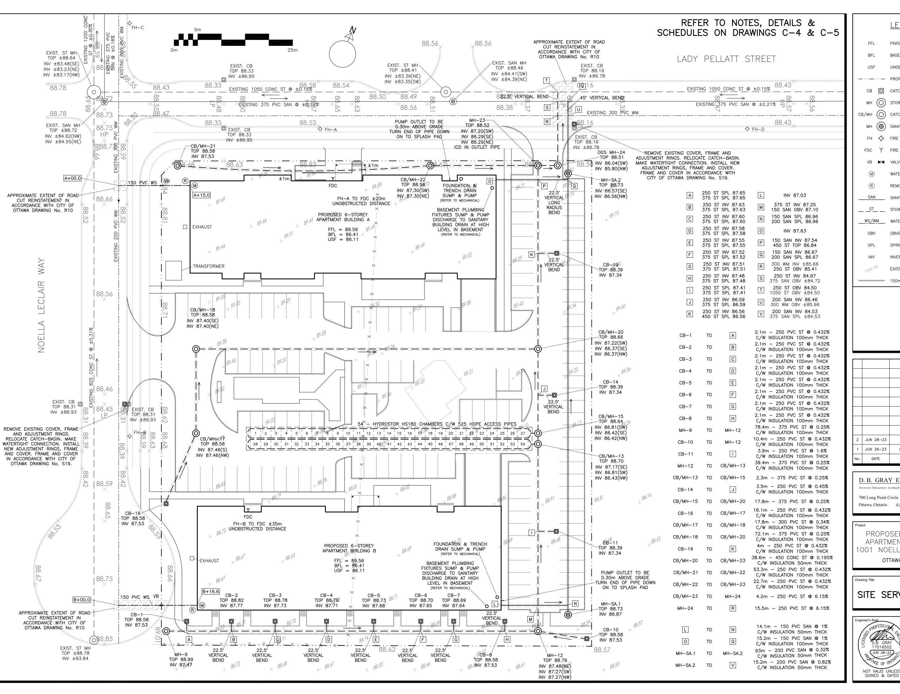
**LEGEND** FINISHED FLOOR ELEVATION BASEMENT FLOOR ELEVATION UNDERSIDE OF FOOTING - · · - PROPERTY LINE CATCH-BASIN MH () STORM MANHOLE CB/MH O CATCH-BASIN/MANHOLE MH ( ) SANITARY MANHOLE FH -O- FIRE HYDRANT FDC Y FIRE DEPARTMENT CONNECTION ■ VALVE & VALVE BOX WATER METER REMOTE WATER METER SANITARY SEWER \_\_\_\_ST\_\_\_ STORM SEWER WS/WM WATER SERVICE/WATERMAIN OBVERT OF PIPE SPRINGLINE OF PIPE INVERT OF PIPE EXISTING GRADE ELEVATION 150mm BARRIER CURB
