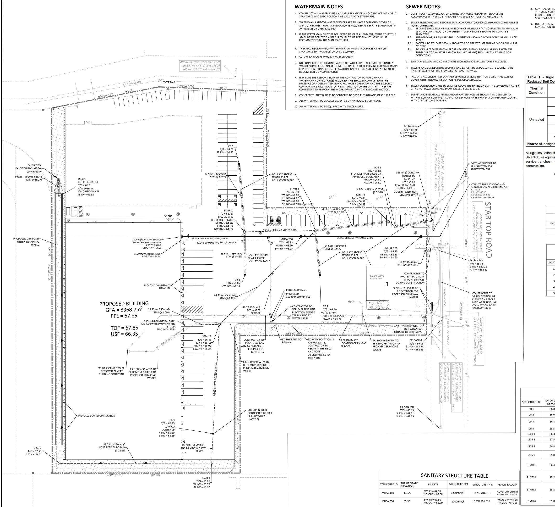
8. CONTRACTOR TO TELEVISE (CCTV) ALL PROPOSED SEWERS ON SITE, OUTLET CONNECTION TO THE MAIN AND PIPES 150mmØ OR GREATER PRIOR TO BASE COURSE ASPHALT. UPON COMPLETION OF CONTRACT, THE CONTRACTOR IS RESPONSIBLE TO FLUSH AND CLEAN ALL SEWERS & APPURTENANCES.
