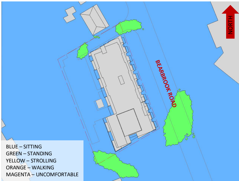
FIGURE 3B: SUMMER – WIND COMFORT, GRADE LEVEL
