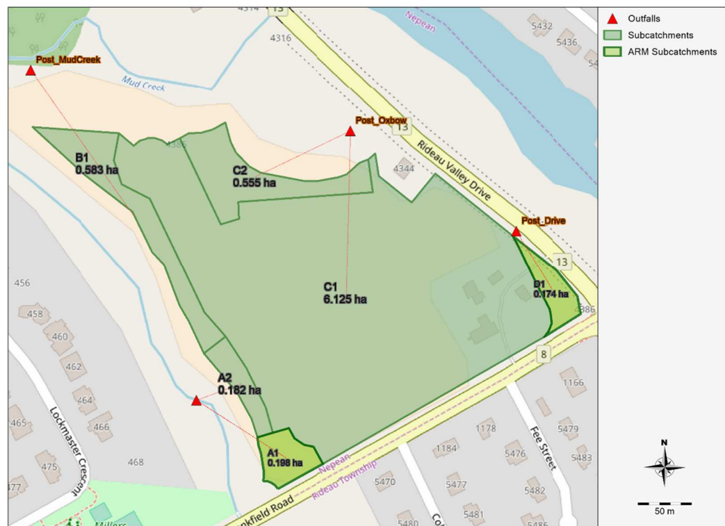
Figure 2: PCSWMM Model Schematic - Proposed Conditions
