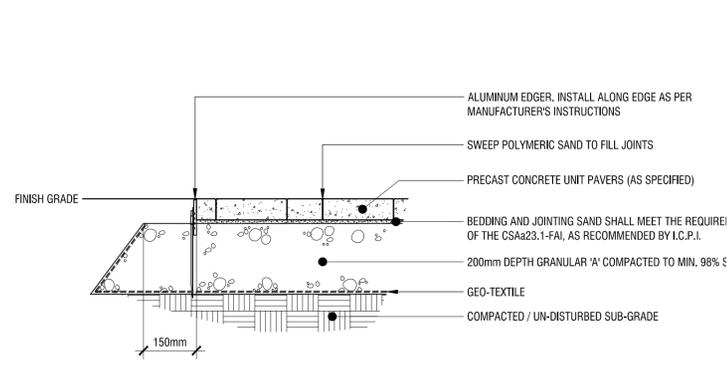
**5** **PRECAST CONCRETE PAVER DETAIL AND LAYOUT**
