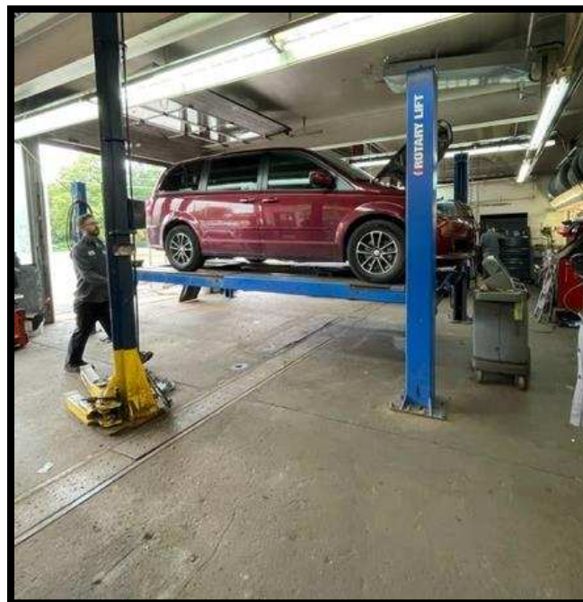
Photograph 10: Another interior view of the garage and oil-water separator channel.
