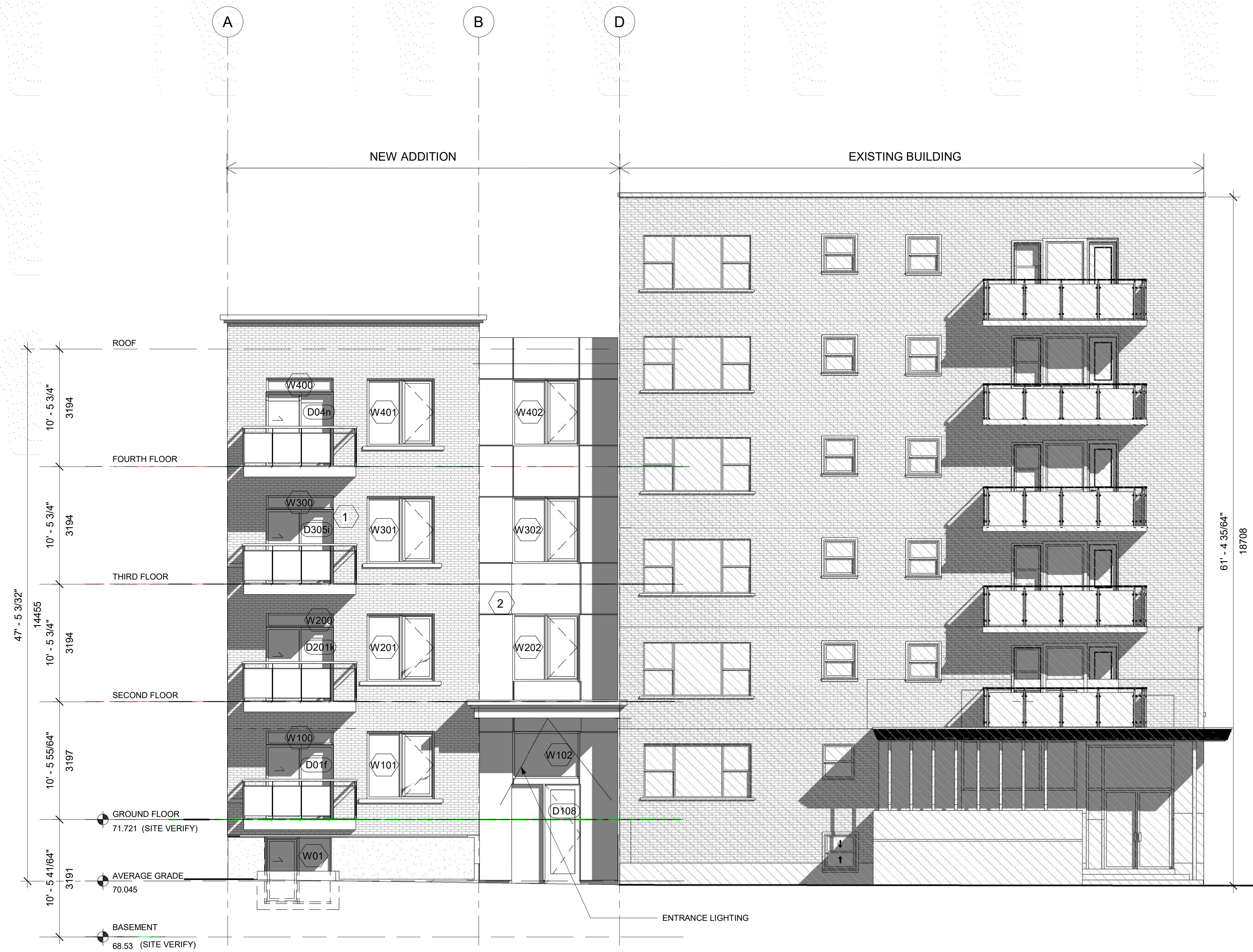
1 Front (North) Elevation 3/16" = 1'-0"
