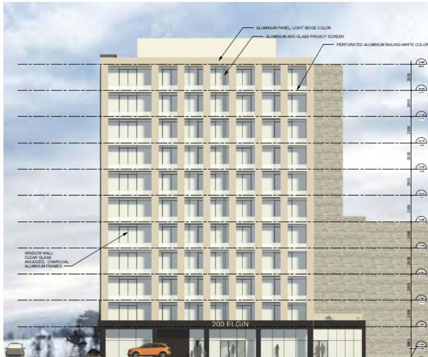
Figure 10: Elgin Street elevation which depicts the proposed inset balconies for the new residential units above the ground floor.
