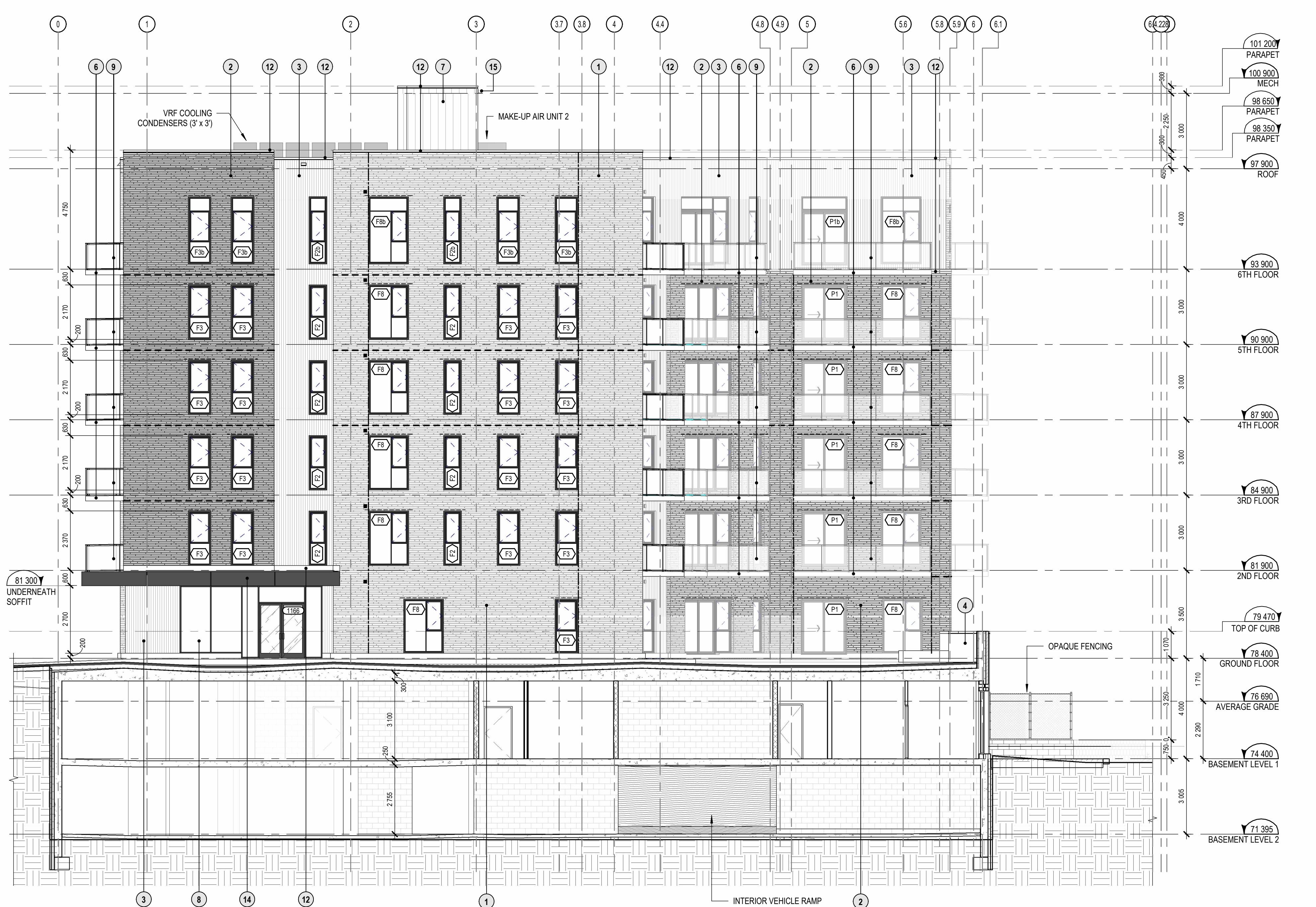
EAST ELEVATION - BUILDING "A" 1:100
