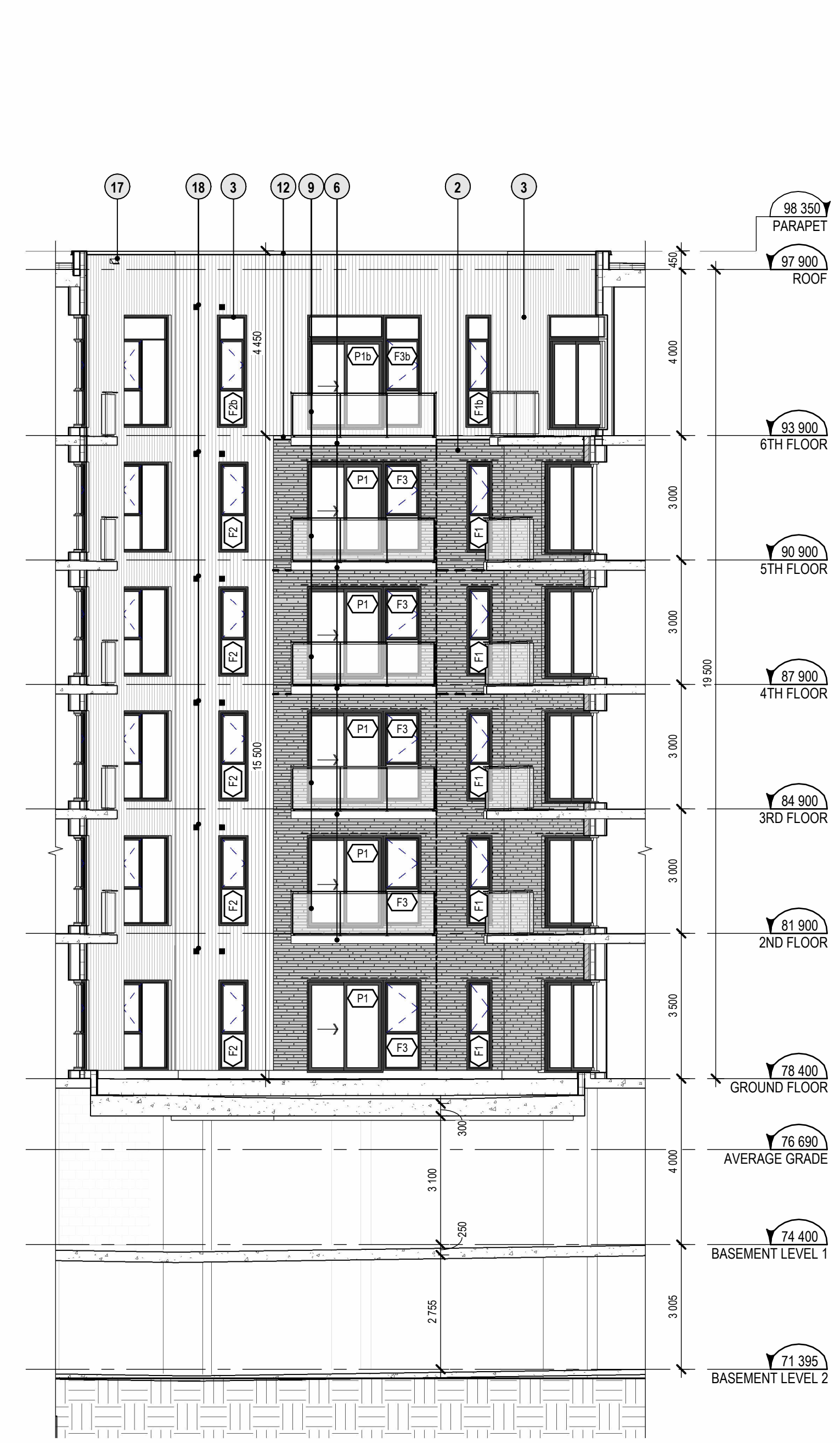
NORTH-WEST CORNER ELEVATION - BUILDING "A" 1:100
