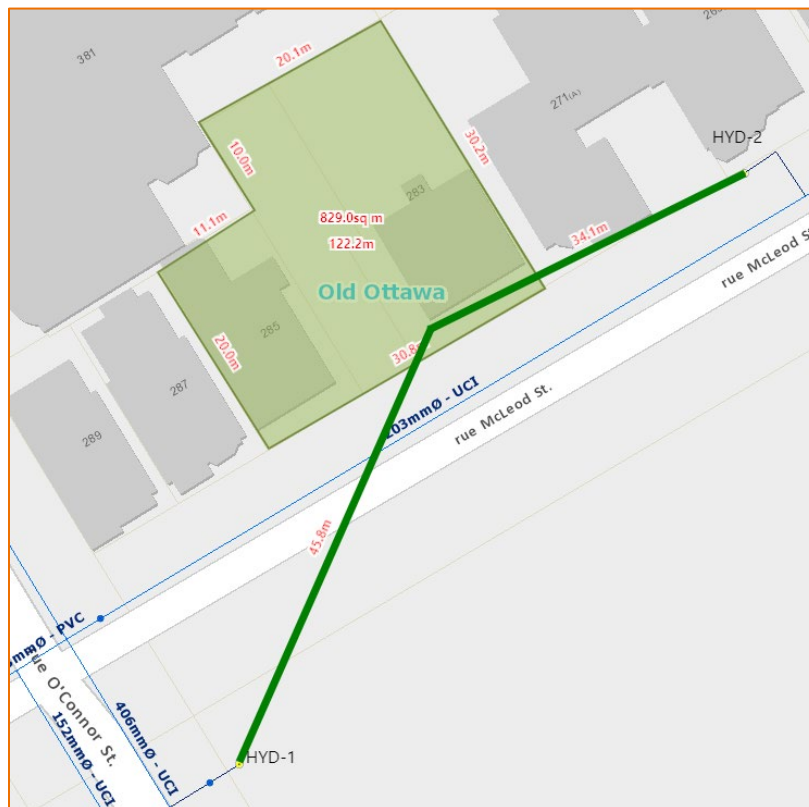
Figure 3.1: Existing Fire Hydrant Coverage Map
