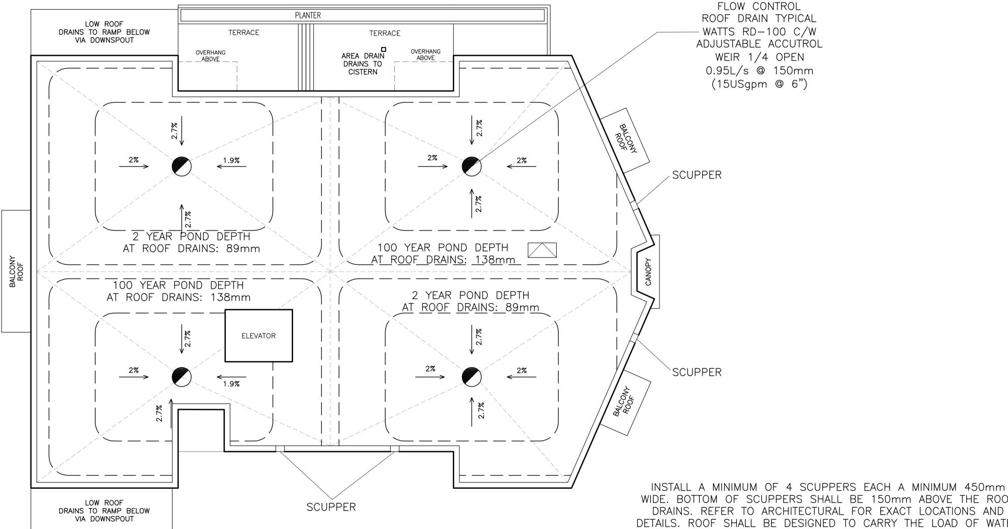
WIDE. BOTTOM OF SCUPPERS SHALL BE 150mm ABOVE THE ROOF DRAINS. REFER TO ARCHITECTURAL FOR EXACT LOCATIONS AND DETAILS. ROOF SHALL BE DESIGNED TO CARRY THE LOAD OF WATER HAVING A 50mm DEPTH AT SCUPPERS (i.e. 200mm DEPTH AT THE ROOF DRAINS). REFER TO STRUCTURAL.
