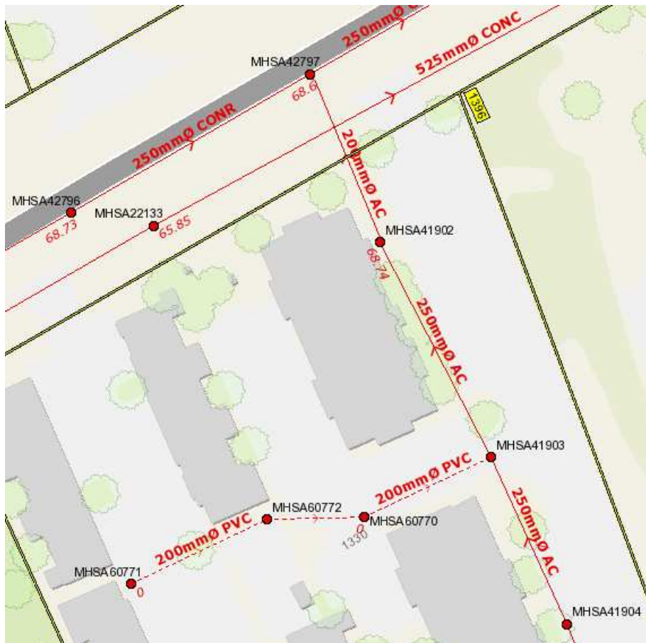
Figure 3: GeoOttawa Existing Sanitary Services
