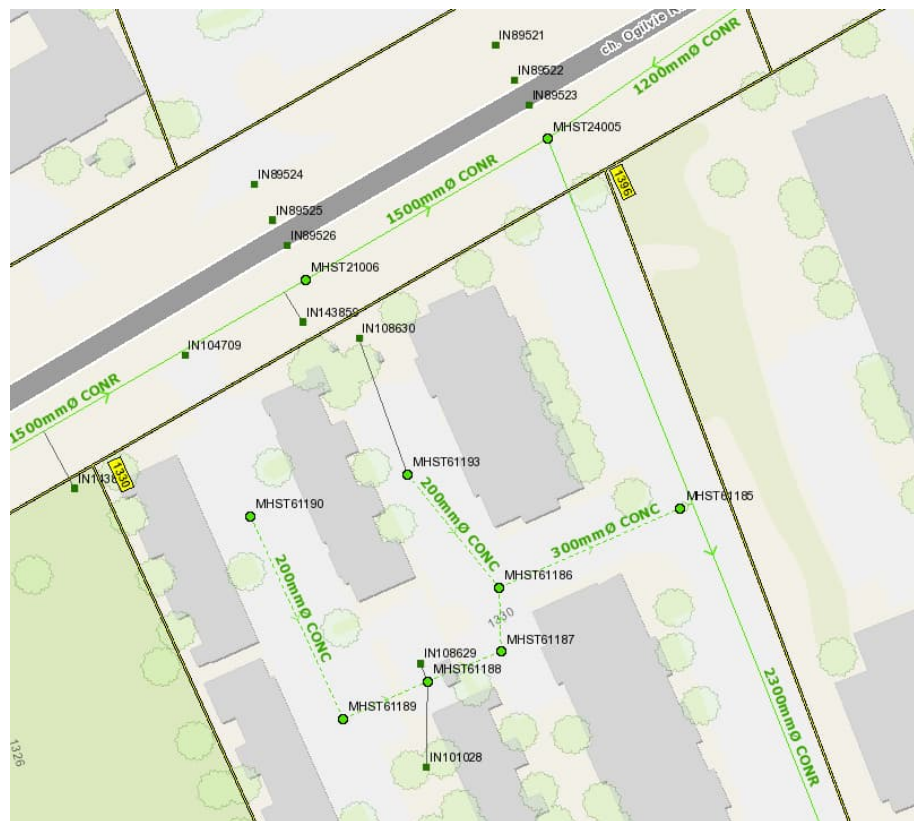
Figure 4: GeoOttawa Existing Storm Services
