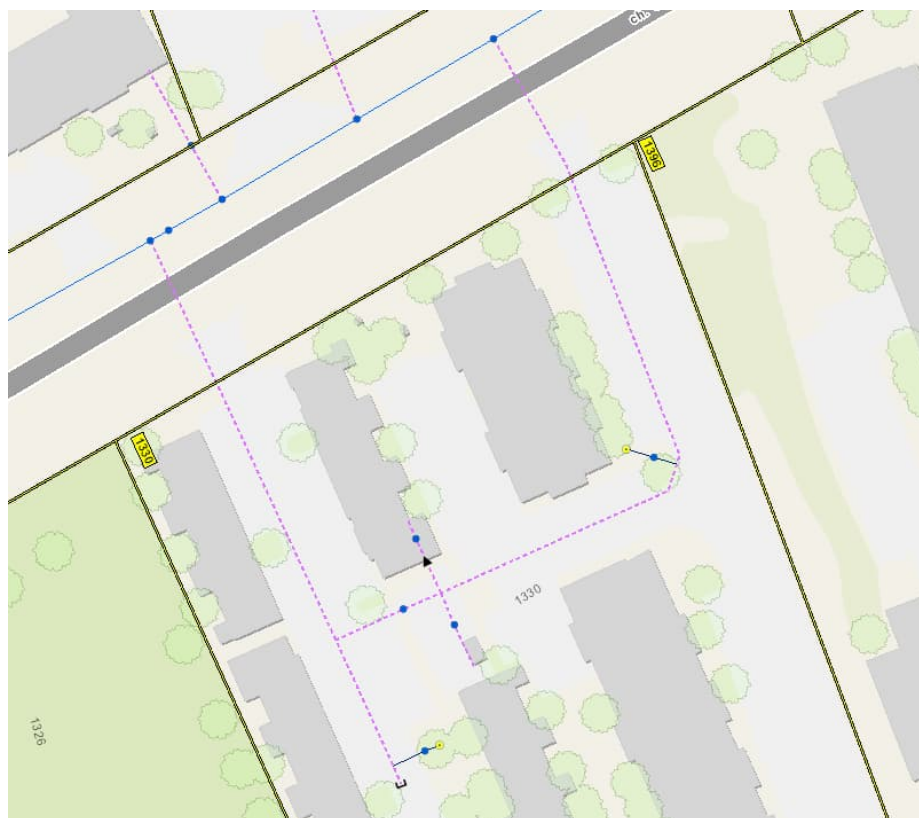
Figure 2: GeoOttawa Existing Water Services
