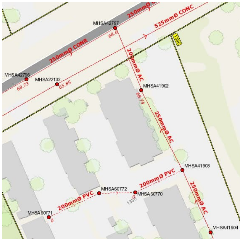
Figure 3: GeoOttawa Existing Sanitary Services
