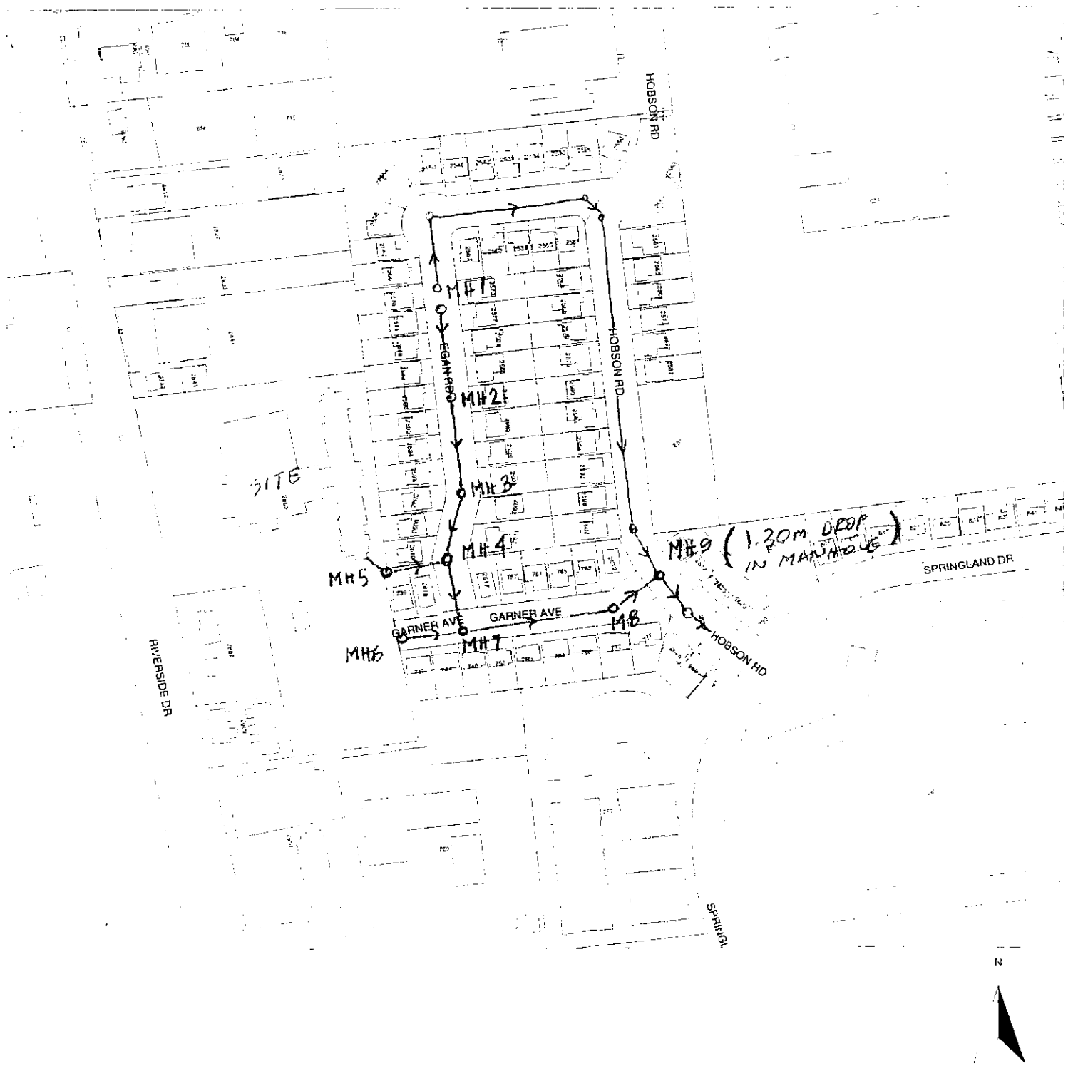
FIGURE 2 EXISTING SITE AND SANITARY SEWERS
