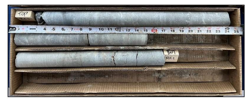
Photograph of Rock Core obtained from BH 2-24 from interval RC1
