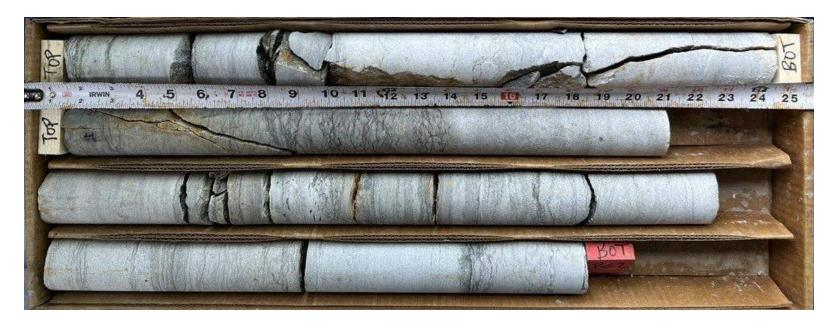
Rock Core RC1 interval ranged between 22'11" to 24'9"; Rock Core RC2 interval ranged between 24'9" to 29'9"
