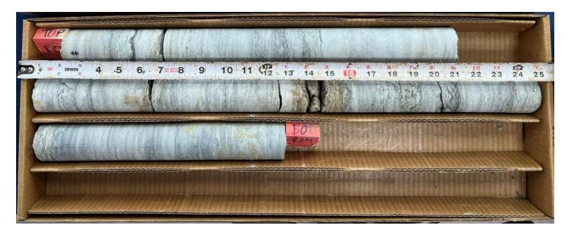
Rock Core interval ranged between 34'10" to 39'9"
