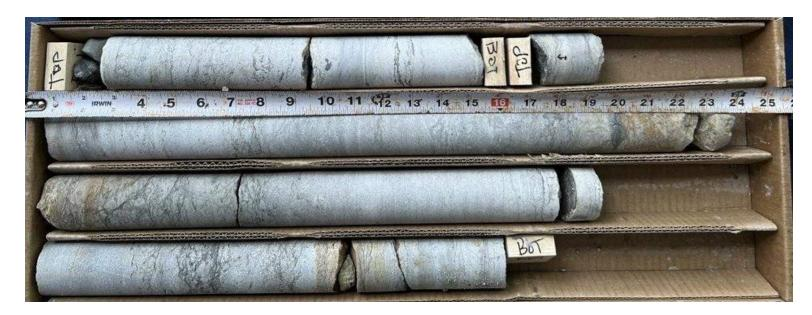
Rock Core RC1 interval ranged between 23'8" to 24'9"; Rock Core RC2 interval ranged between 24'9" to 29'9"
