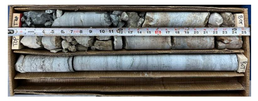
Rock Core RC1 interval ranged between 19'11" to 24'11"; Rock Core RC2 interval ranged between 24'11" to 29'10"
