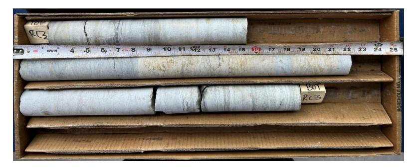
Rock Core interval ranged between 29'7" to 34'4"
