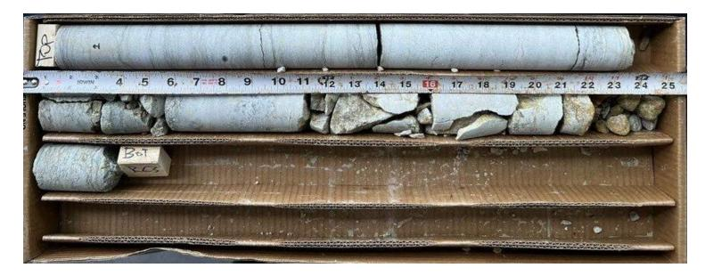
Rock Core interval ranged between 29'9" to 34'9"
