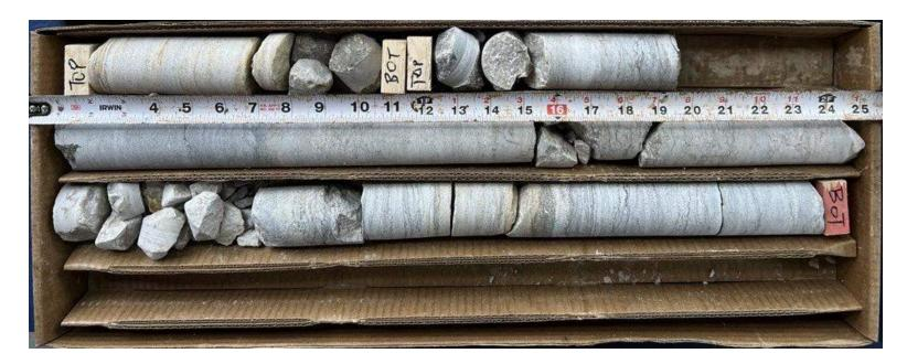
Rock Core RC1 interval ranged between 4'9" to 6'9"; Rock Core RC2 interval ranged between 24'4" to 29'8"
