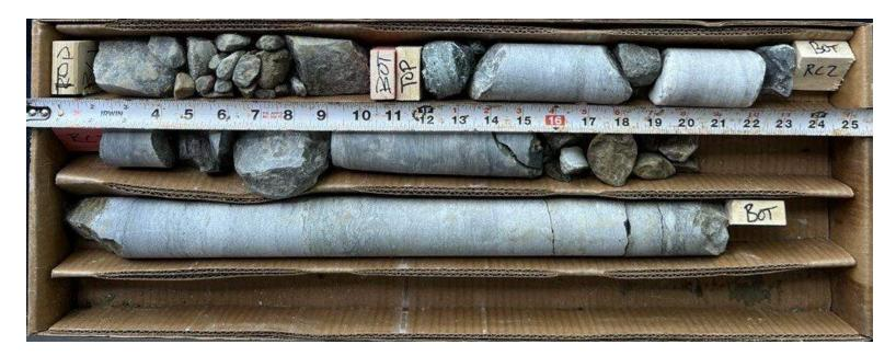
Rock Core RC1 interval ranged between 3'11" to 6'6"; Rock Core RC2 interval ranged between 12'11" to 14'6"; Rock Core RC3 interval ranged between 20'11" to 24'10"
