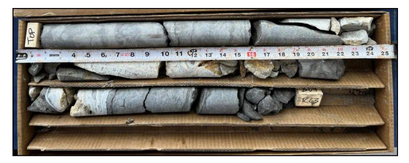
Photograph of Rock Core obtained from BH 1-24 from interval RC3
