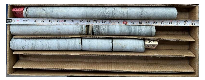
Rock Core interval ranged between 29'10" to 34'9"
