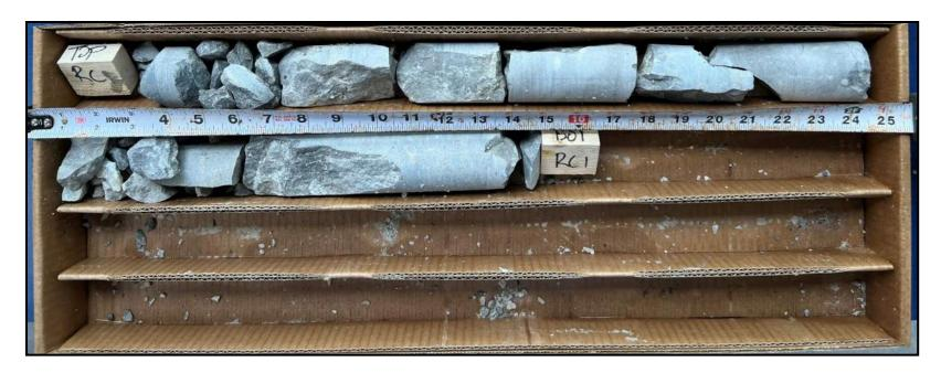
Photograph of Rock Core obtained from BH 3-24 from interval RC1
