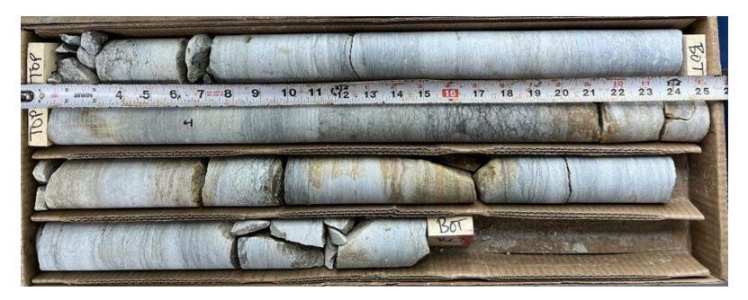
Rock Core RC1 interval ranged between 22'5" to 24'9"; Rock Core RC2 interval ranged between 24'9" to 29'6"
