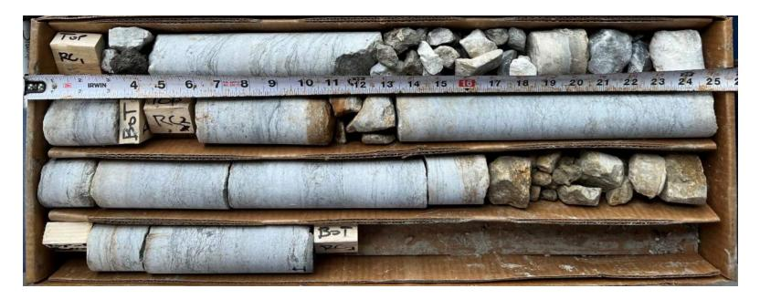
Rock Core RC1 interval ranged between 20'2" to 24'11"; Rock Core RC2 interval ranged between 24'11" to 29'7"
