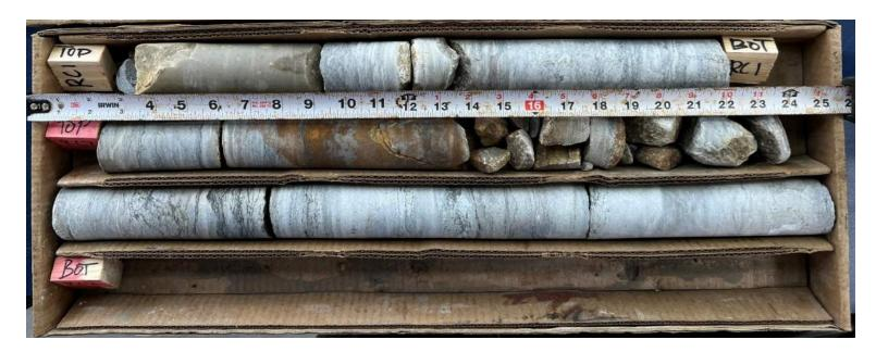
Rock Core RC1 interval ranged between 21'10" to 25'0"; Rock Core RC2 interval ranged between 25'0" to 29'11"
