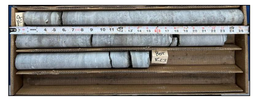
Photograph of Rock Core obtained from BH 2-24 from interval RC3
