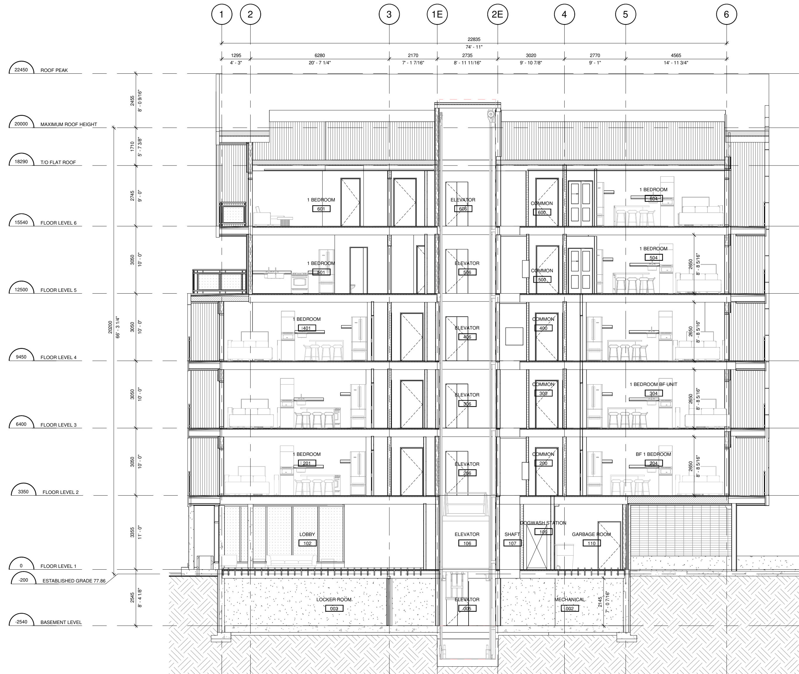
1 SECTION THRU ELEVATOR A302 1:100
