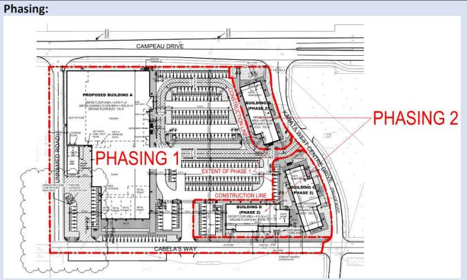
The proposed development will be constructed in two phases. Phase 1 will include Building A and parking lot, except 25 parking spaces which will be constructed in Phase 2 with Building B, C, D. Depending on the sales situation, Phase 2 may directly commence following Phase 1. Either way, phasing construction will not cause shortage of parking spaces.
