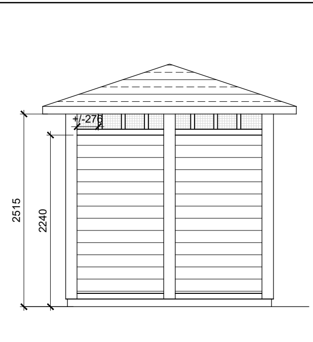
3 GARBAGE ENCLOSURE A-100 REAR ELEVATION SCALE = 1 : 50
