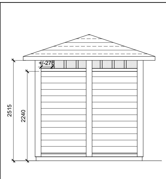
3 GARBAGE ENCLOSURE REAR ELEVATION SCALE = 1 : 50
