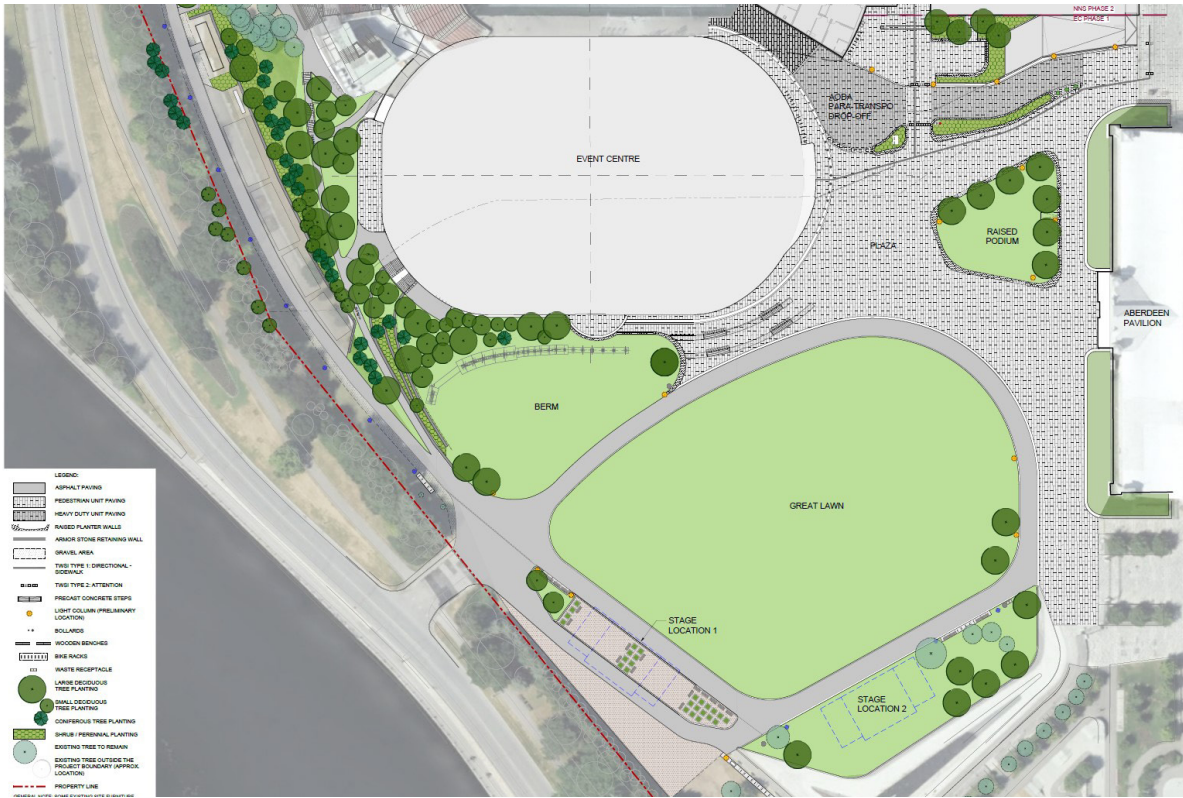
Proposed landscape plan showing the new path geometry, vegetation strategy and paving design (CSW, 2025).
