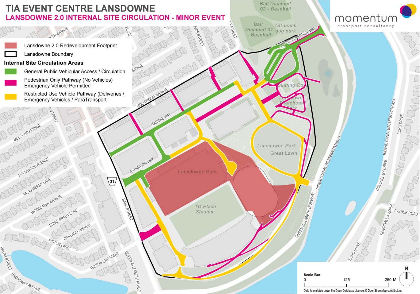
Figure 4.2: Lansdowne 2.0 Internal Site Circulation Plan (Minor Events)
