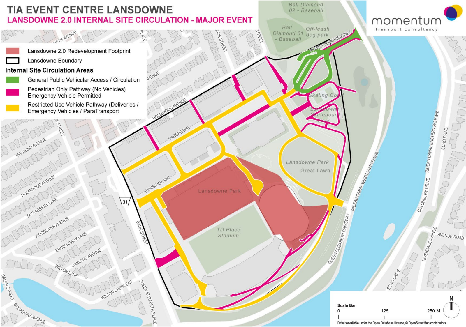
Figure 4.3: Lansdowne 2.0 Internal Site Circulation Plan (Major Events)
