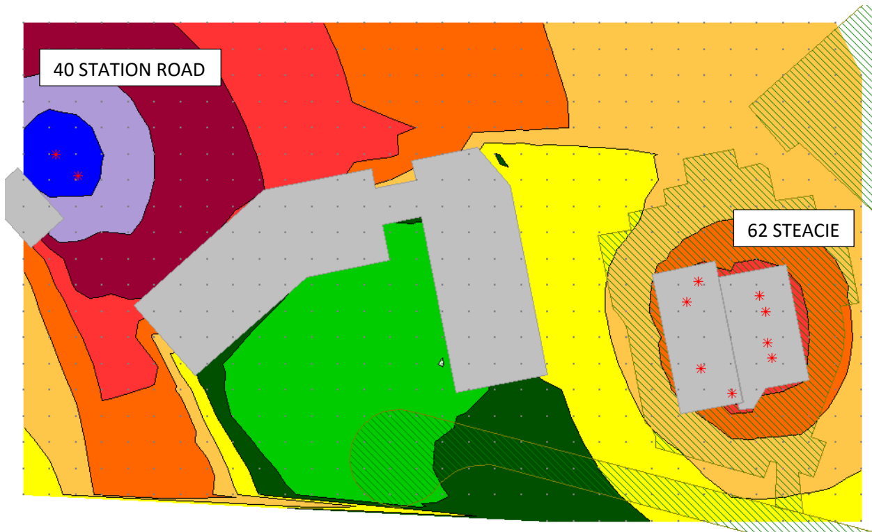
FIGURE 6: STATIONARY NOISE CONTOURS – DAYTIME PERIOD (10.5 METRES ABOVE GRADE)
