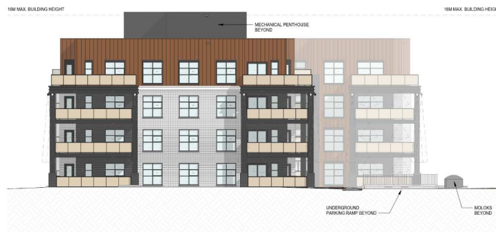
Figure 12v.2 – North elevation (August 2024).
