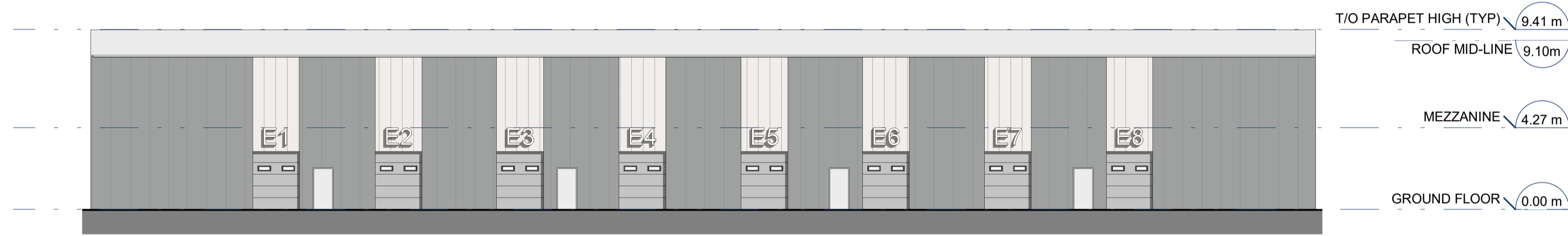
E2 BUILDING E - EXTERIOR ELEVATION (NORTH) E400 1 : 200
