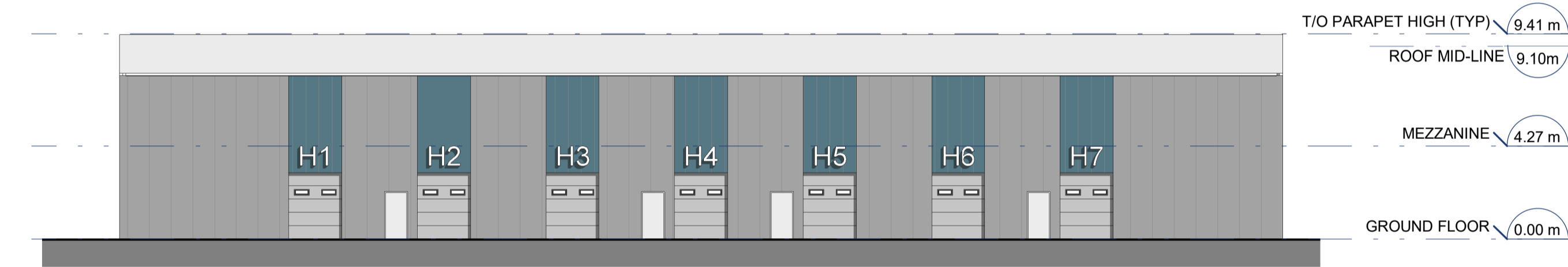
H2 BUILDING H - EXTERIOR ELEVATION (NORTH) H400 1 : 200
