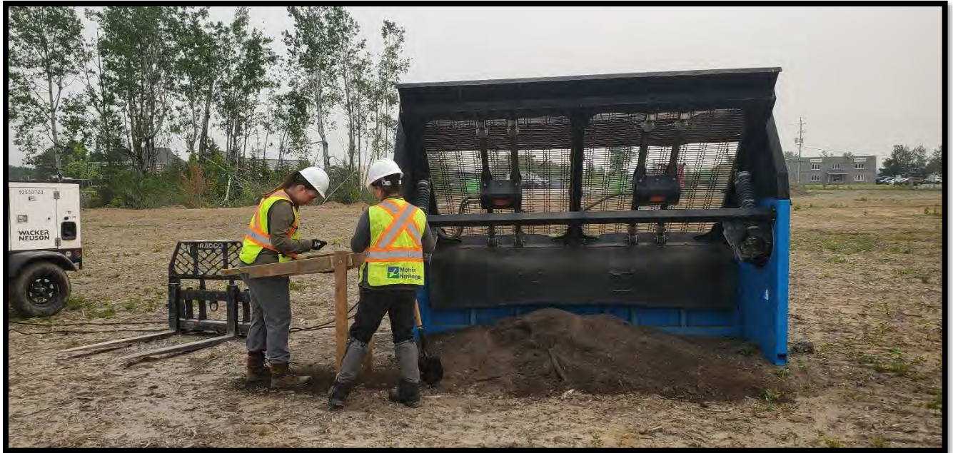
Figure 19: Mechanical sample screening in progress. (MH1174-D096)
