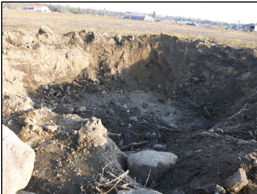
Image 12. Open test hole showing the depth of added fill in the southern half of the property, facing southeast. (PR16-42D044)
