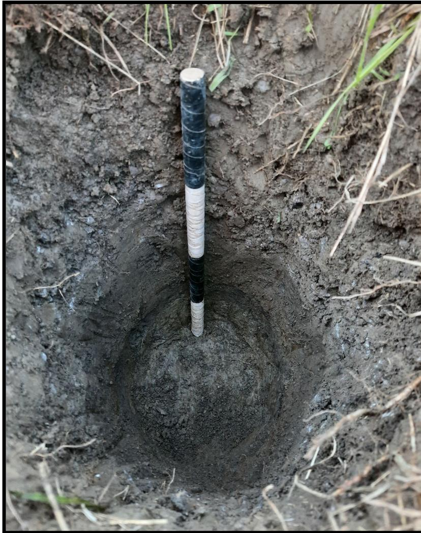
**Figure 12: Typical test pit (MH1313-D01).**
