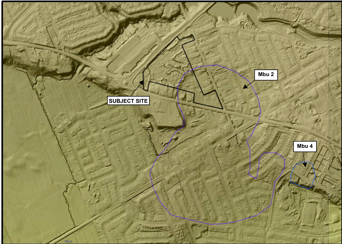
Figure 1 – LiDAR Image of Subject Site and closest documented landslides.
