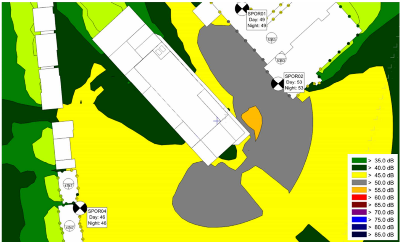
Figure 4: Noise modelling results, emergency generator operation (with mitigation).
