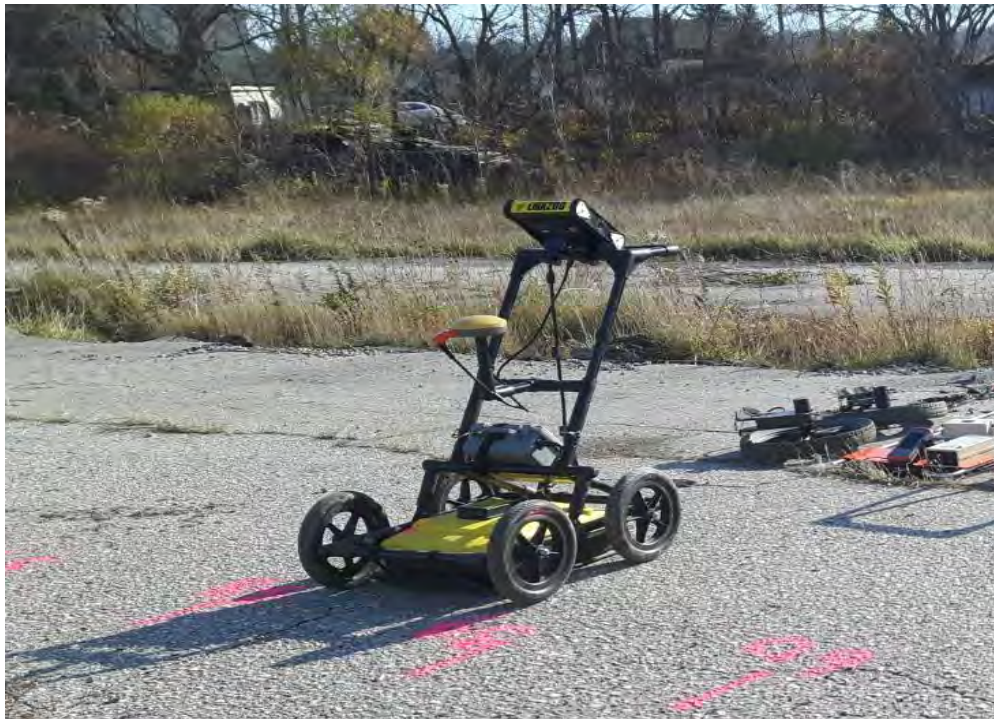
Figure 3: Typical GPR Acquisition System Setup
