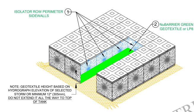
STEP 1: INSTALL ISOLATER ROW PERIMETER SIDEWALLS AND ATTACH GEOTEXTITLE TO THEM.
