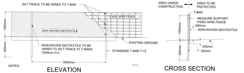
SILTATION CONTROL FENCE TO BE TERRAFIX TERRAFENCE, OR EQUIVALENT, OR CONSTRUCTED AS INDICATED BELOW.
