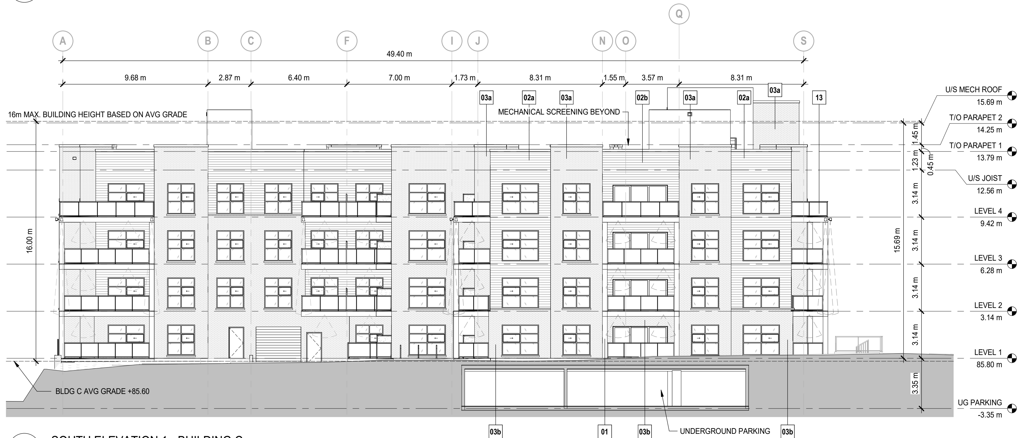
2 SOUTH ELEVATION 1 - BUILDING C DP30-02-02 SCALE: 1 : 150
