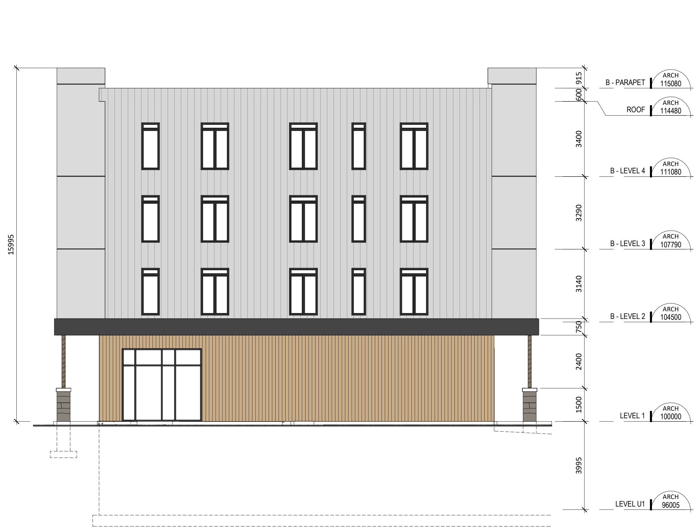
2 RIGHT ELEVATION - BUILDING B A302 1 : 100
