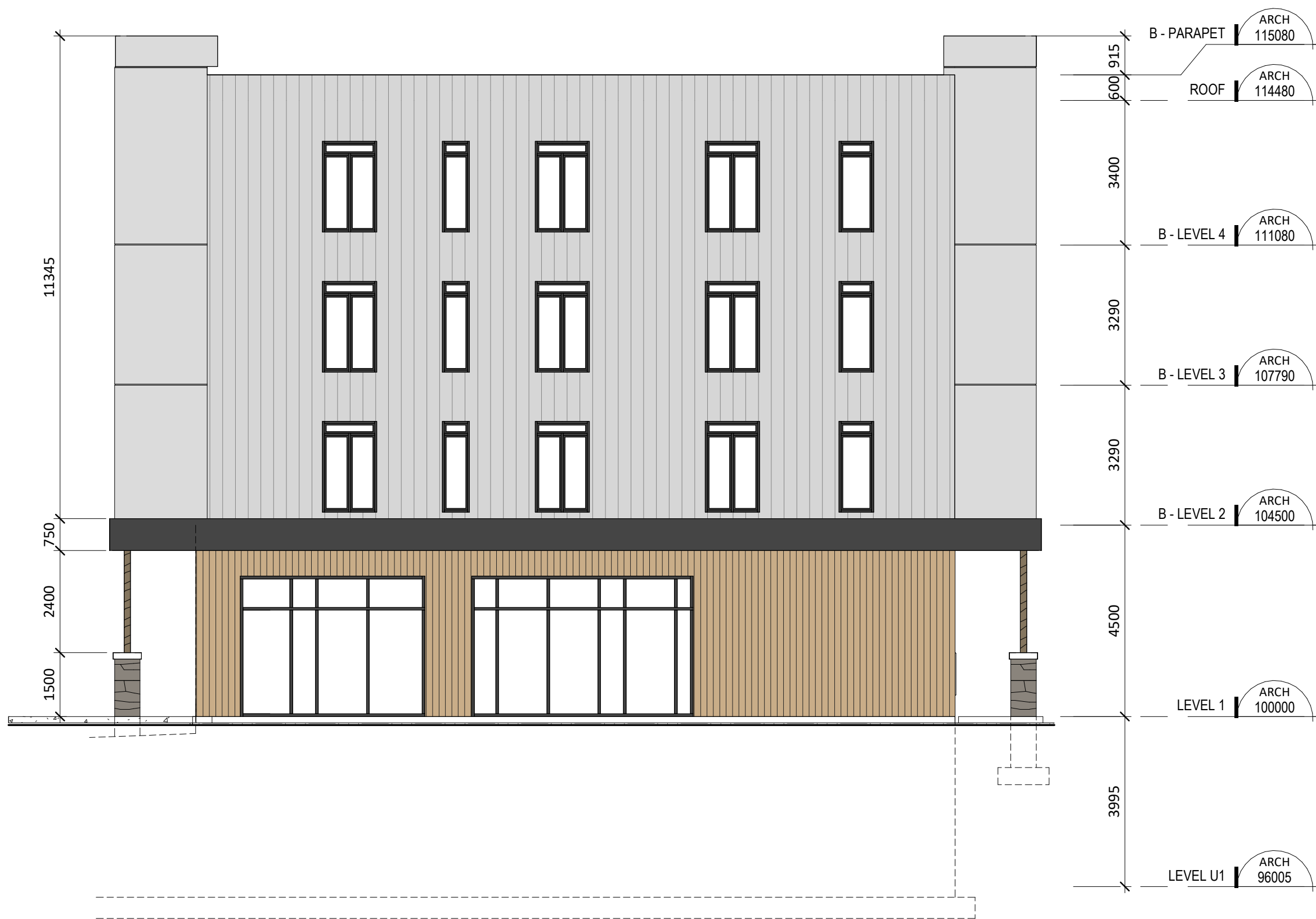
3 LEFT ELEVATION - BUILDING B A302 1 : 100
