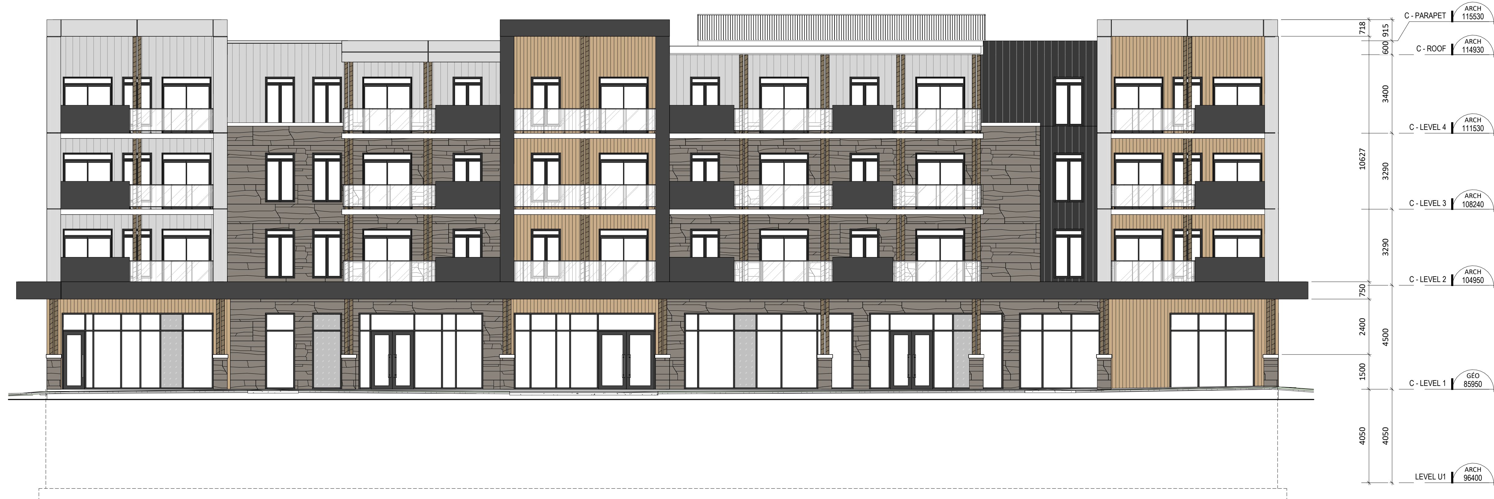
1 EAST ELEVATION - BUILDING C A202 1:100
