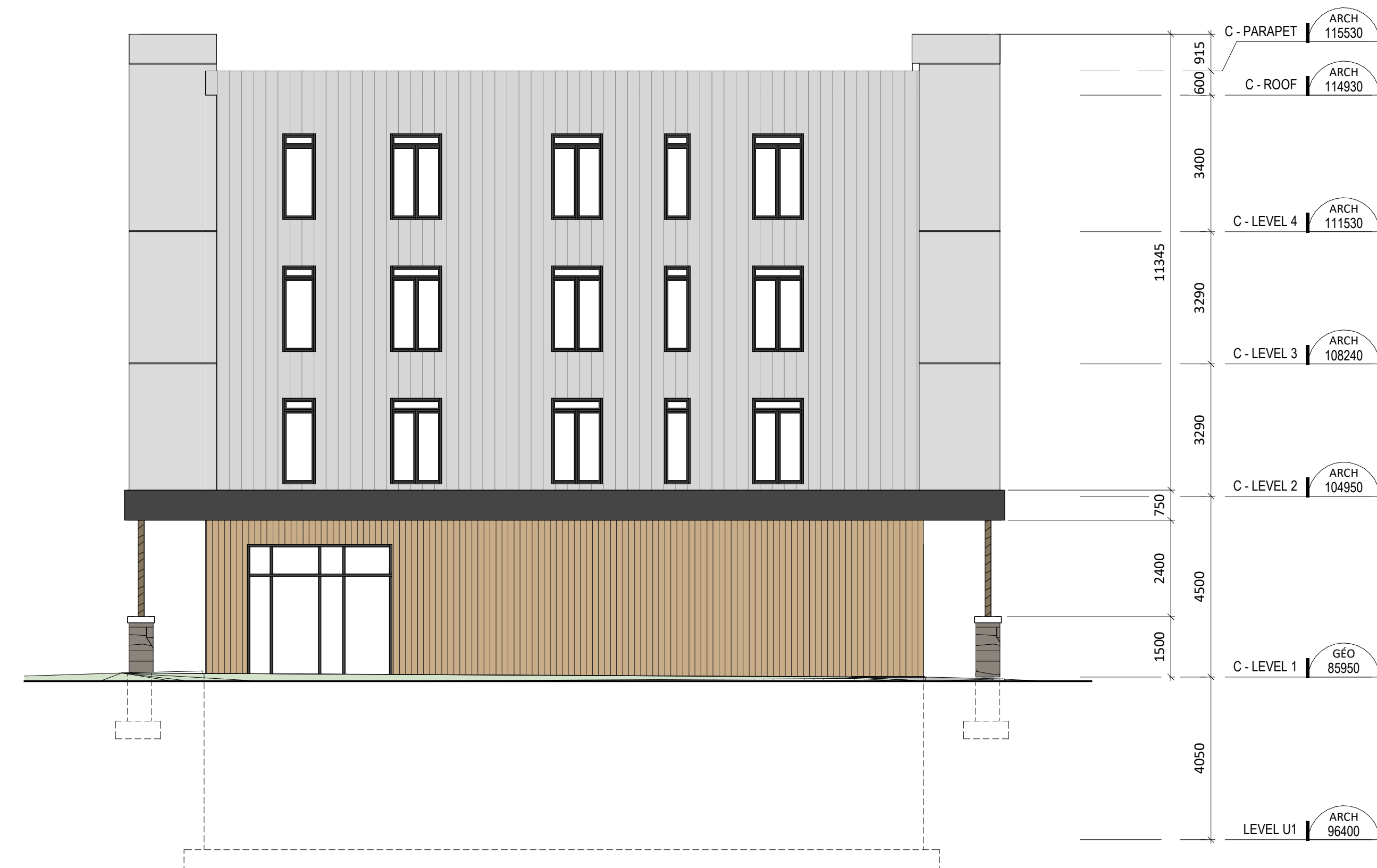
2 NORTH ELEVATION - BUILDING C A202 1:100
