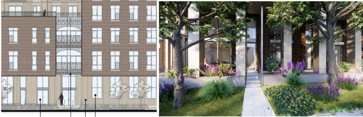
Figure 15: Detail view of the main entrance at Blackburn and ground floor entrances along Blackburn, defining the cadence along the street. Salvaged limestone from Bate Hall has been used as a facing of ground floor terraces along Blackburn. The reuse provides a link to the existing building and integrates the two facades.
