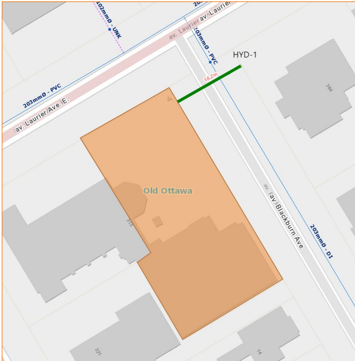
Figure 2.1: Existing Fire Hydrant Coverage
