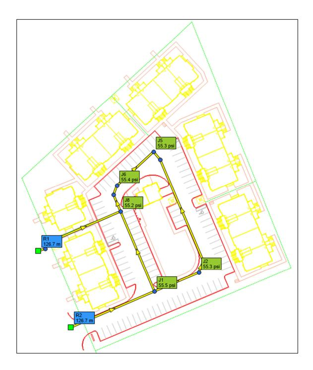
Figure 3.4 Minimum Pressures (psi) During PKHR Conditions
