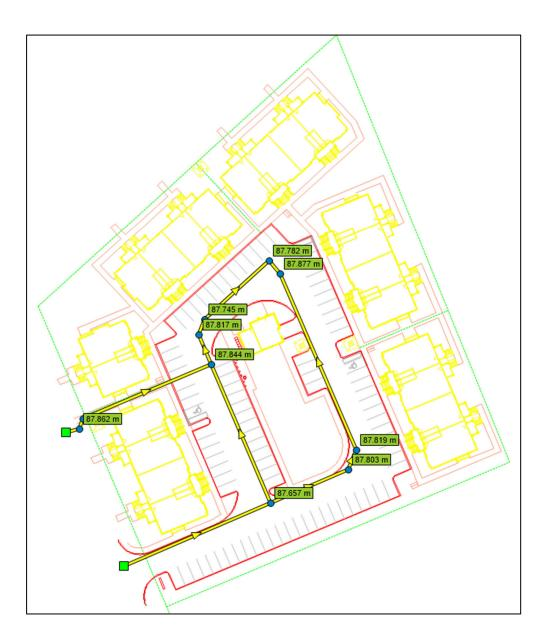
Figure 3.2 Ground Elevations (m) at Nodes
