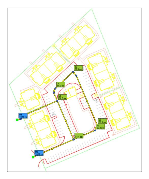
Figure 3.3 Maximum Pressures (psi) During AVDY Conditions
