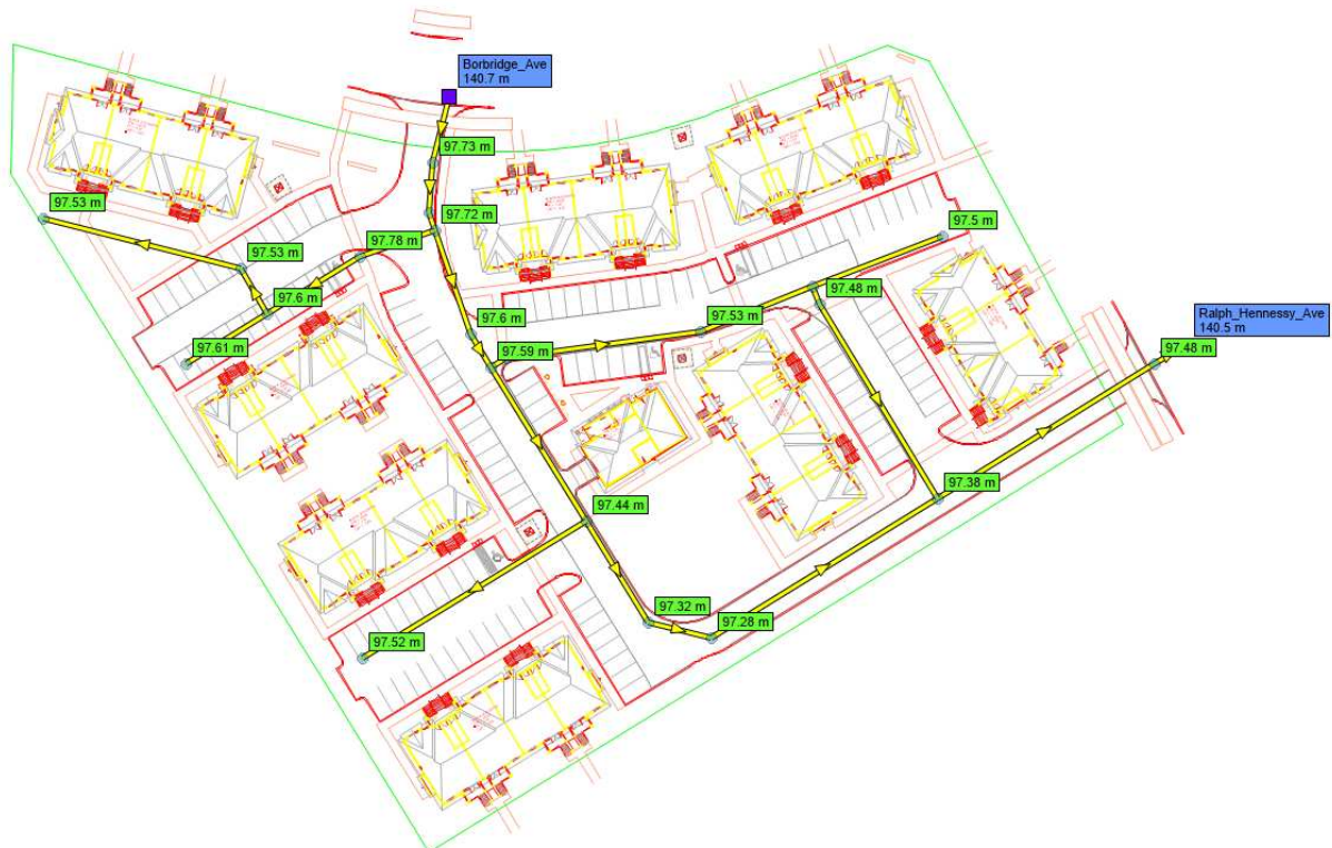
Figure 3.2 Ground Elevations (m) at Nodes
