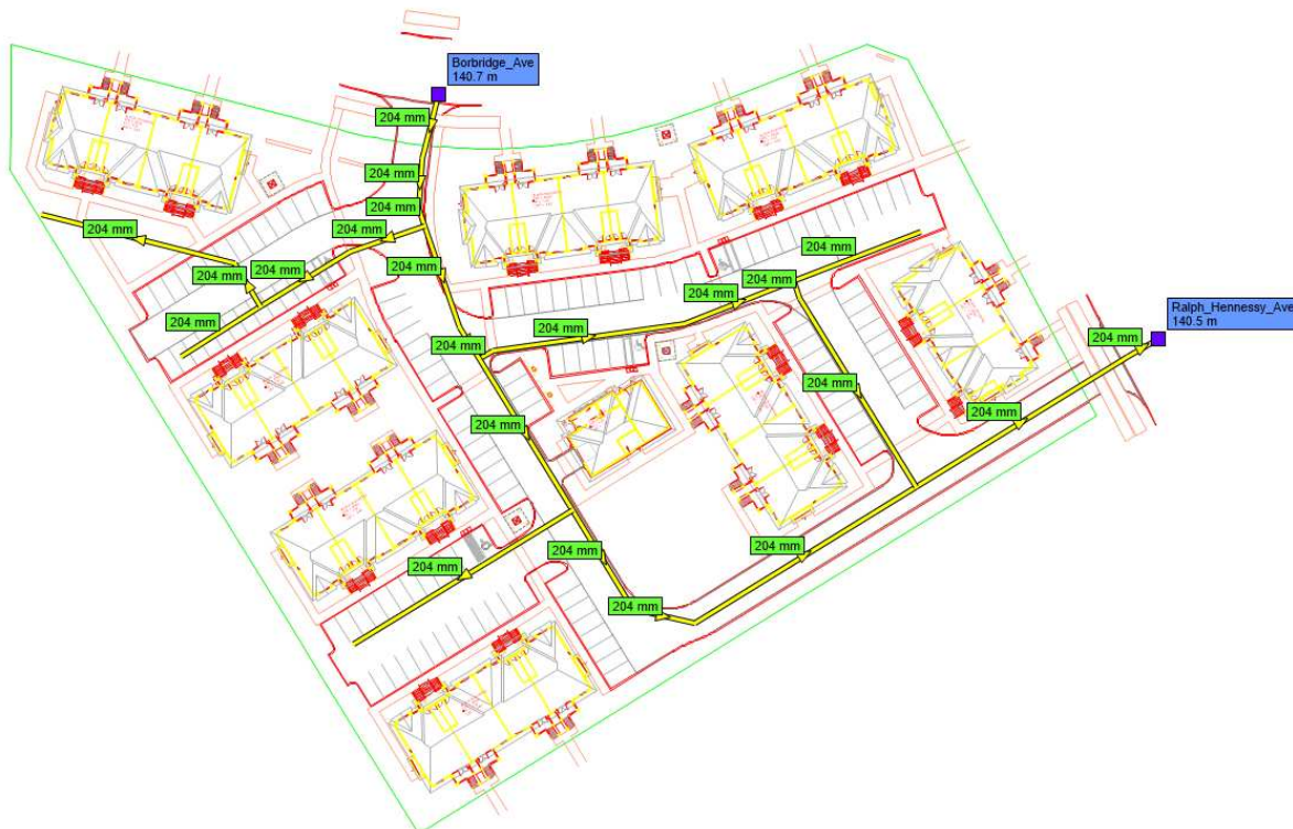
Figure 3.1 Proposed Watermain Layout and Pipe Diameters (mm)
