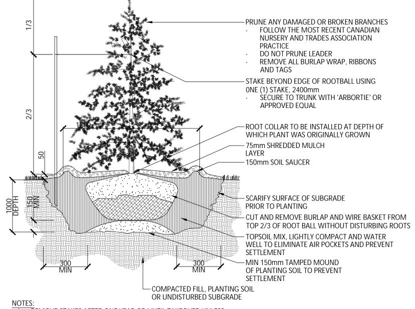
1. REMOVE STAKES AFTER ONE YEAR OR UNTIL TAKEOVER UNLESS OTHERWISE DIRECTED BY THE LANDSCAPE ARCHITECT. 2. TOPSOIL MIXTURE AND SHREDDED MULCH AS PER SPECIFICATION
