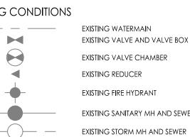
EXISTING SANITARY MH AND SEWER EXISTING STORM MH AND SEWER EXISTING CATCHBASIN MANHOLE EXISTING CATCHBASIN REMOVAL ITEMS ASPHALT/CONCRETE/VEGETATION TO BE REMOVED
