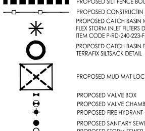
PROPOSED SILT FENCE BOUNDARY AS PER OPSD 219.110 PROPOSED CONSTRUCTIN FENCE AS PER DETAIL. PROPOSED CATCH BASIN MH PROTECTION AS PER FLEX STORM INLET FILTERS DETAIL. ITEM CODE P-RD-240-223-FX PROPOSED CATCH BASIN PROTECTION AS PER
