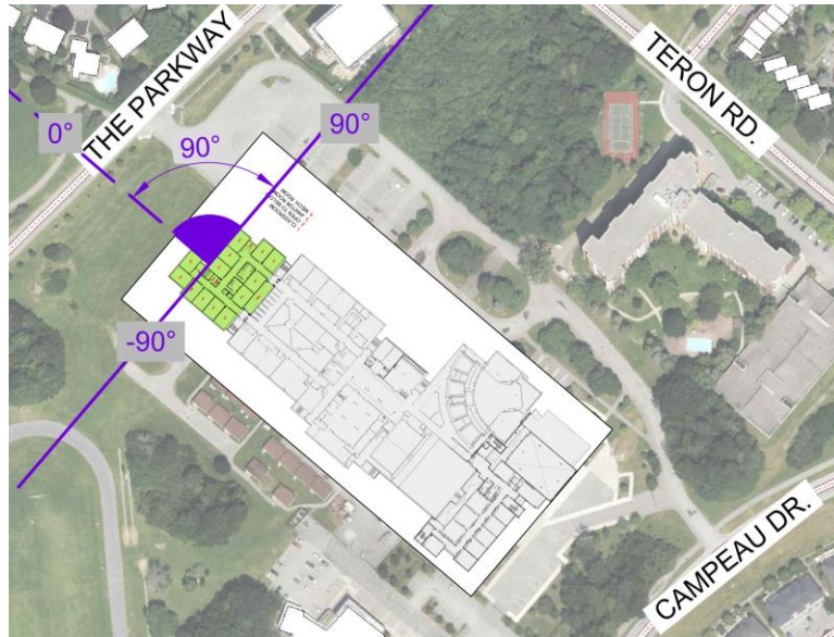
Figure 3.6 – Site plan of EOM showing angles between POR B and The Parkway (angle in purple).
