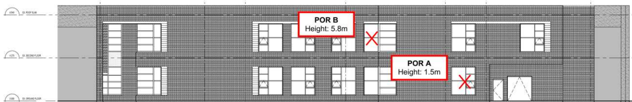
Figure 3.2 –Elevation of Northwest Side of New Addition showing the plane of window (POW) point of reception, with the locations and heights of PORs A and B. The red 'X' denotes the receiver location used in STAMSON.
