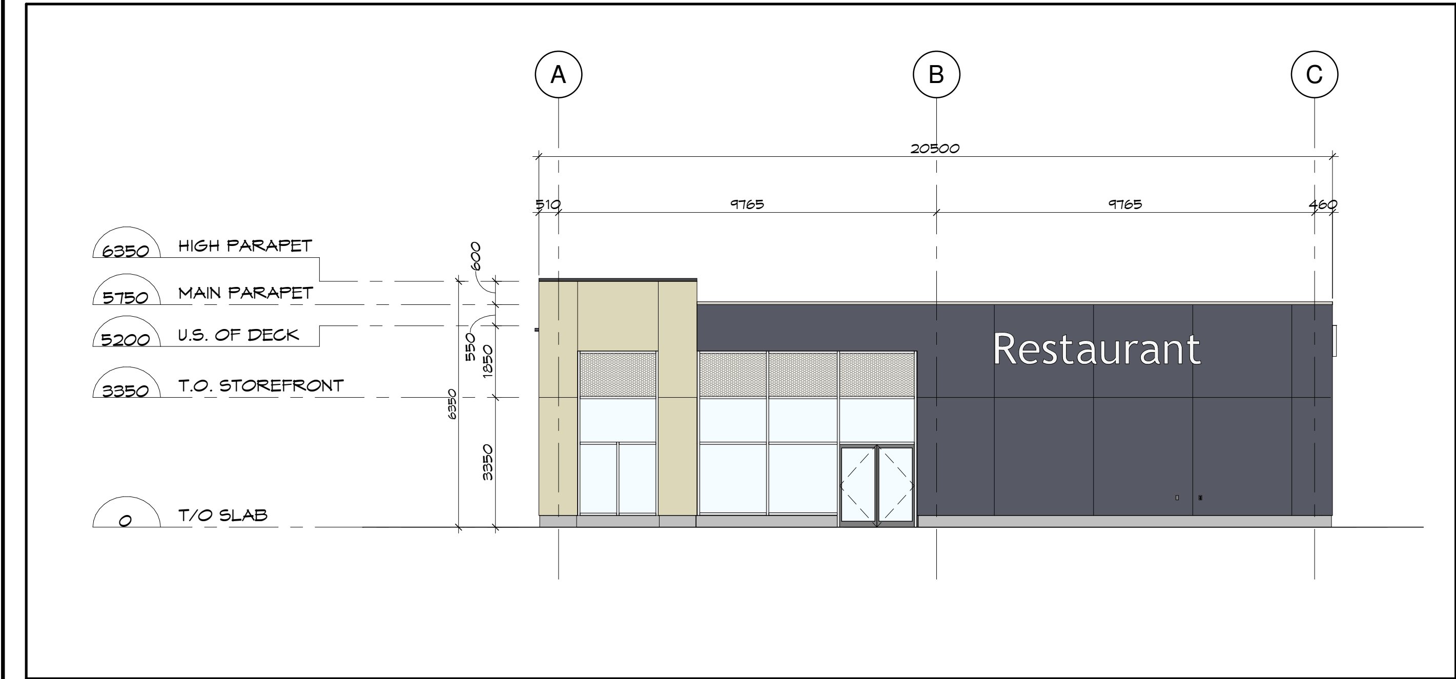
3 SIDE ELEVATION 1 (GRID 6) SP-E SCALE: 1 : 100
