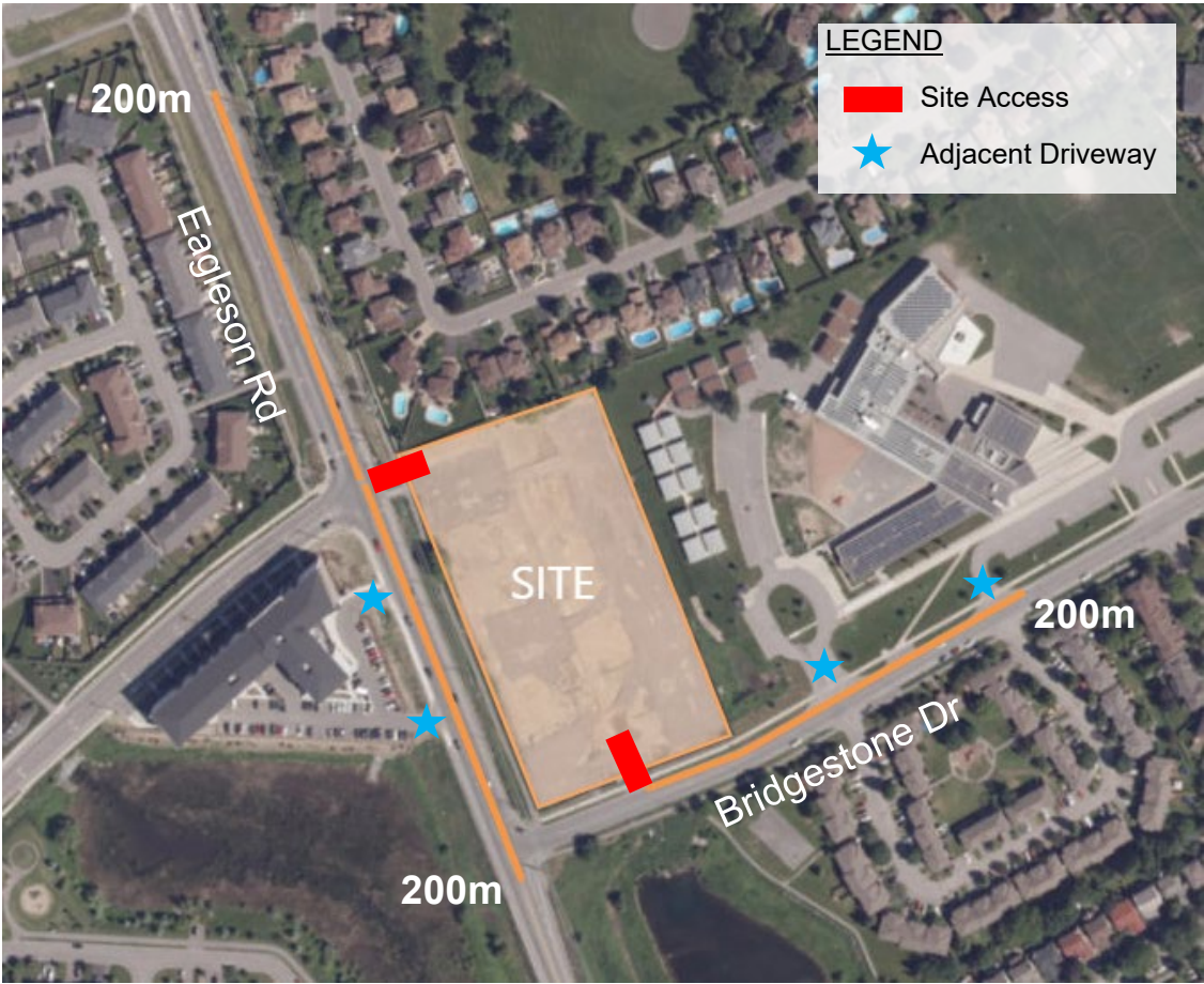
Figure 3-1 Driveways within 200m from Site Access Driveways
