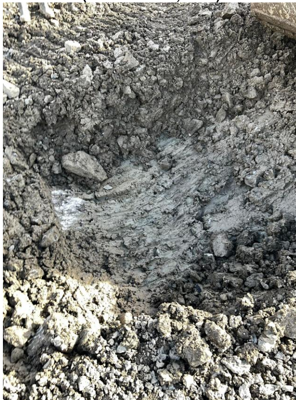
Photo 4: Test Pit Excavated in the clay and boulder fill, wet fill conditions observed (November 23, 2021)
