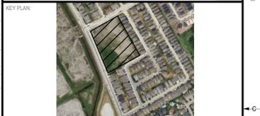
BEARING NOTE: BEARINGS ARE METRIC GRID, DERIVED FROM THE EASTERLY LIMIT OF BLOCK 196 PLAN 44-1640, HAVING A GRID BEARING OF N87°17'E. DISTANCES ARE GROUND AND CAN BE CONVERTED TO GRID BY MULTIPLYING BY THE COMBINED SCALE FACTOR OF 0.9999.
