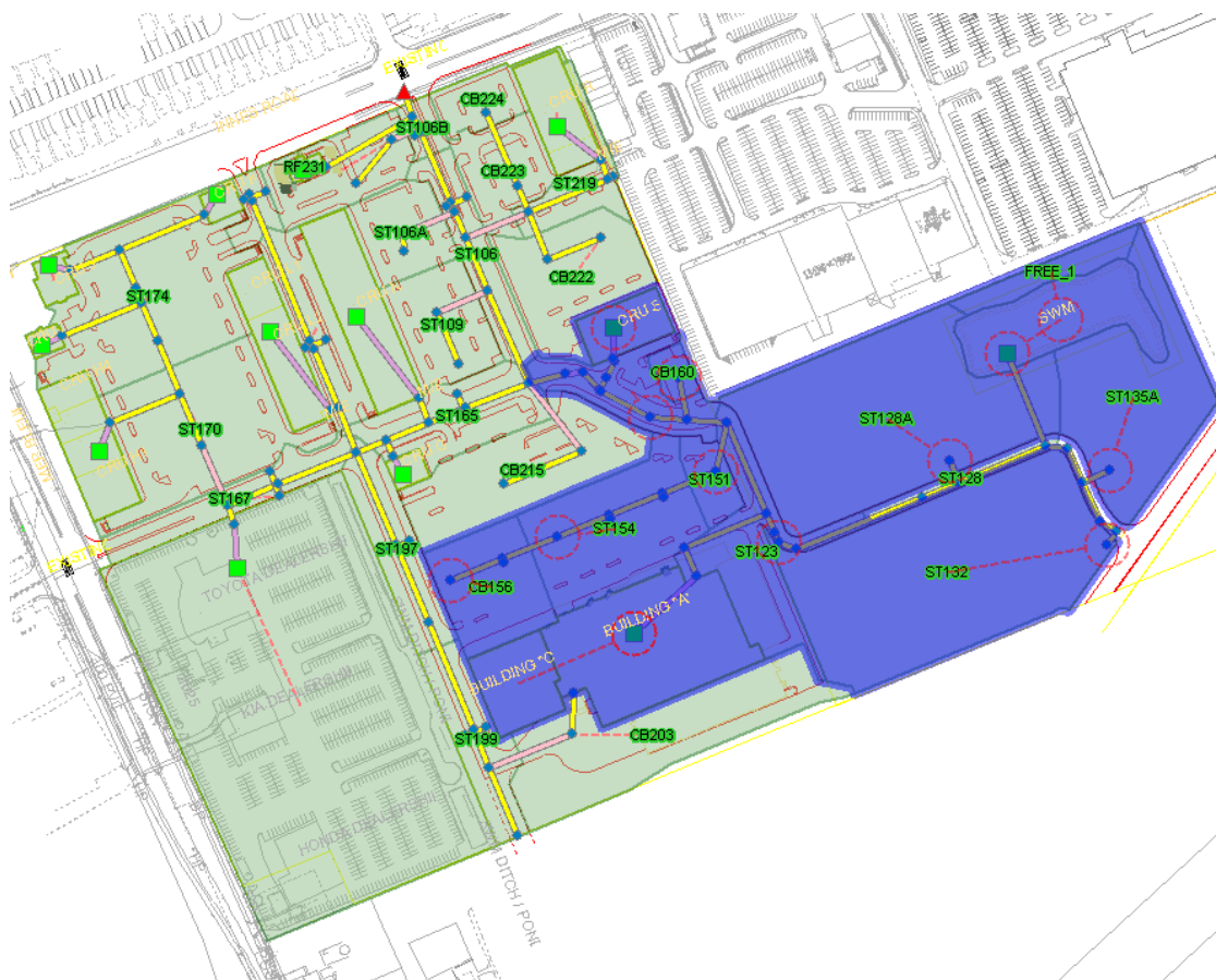
Figure 4.1: PCSWMM Model Subcatchments in light green (area in blue is tributary to the proposed dry pond, area = 9.6 ha)
